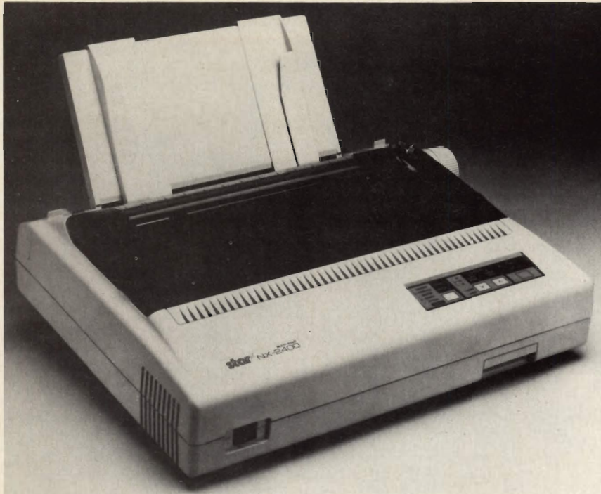
Star's 24-wire NX-2400 Multi-Font offers four resident fonts, 360 by 360 dpi graphic resolution, 170 cps draft mode, and 7K buffer (expandable to 39K).
